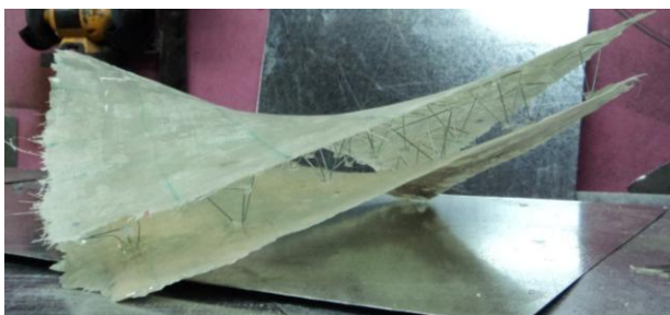
Fig. 38. Sandwich Panel W3-i. Tetrahedrons core paraboloid.
