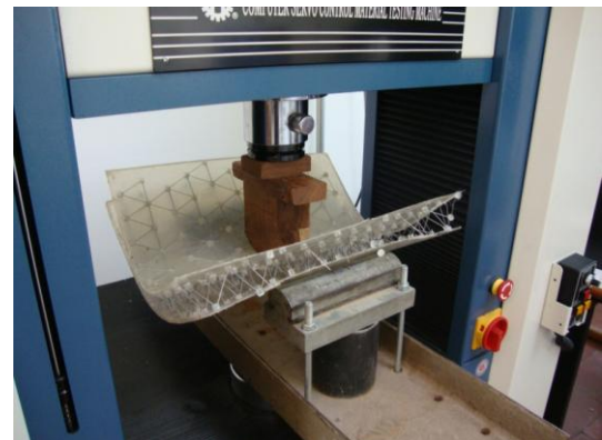
Fig. 30. Bending test sandwich panel W3-i. Invested closed.
