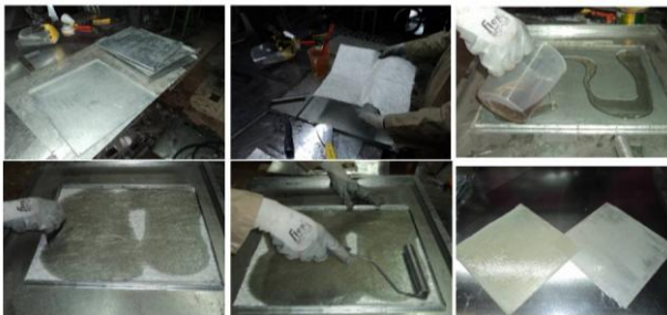
Fig. 19. Manufacturing test panels W3-i.
