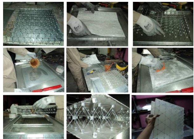
Fig. 21. W3i panel manufacturing.
