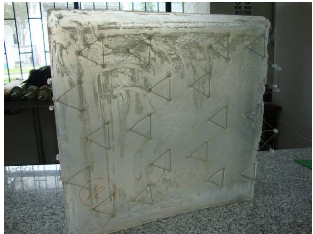
Fig. 26. Sandwich Panel W3-i. Half cuboctaedros.
