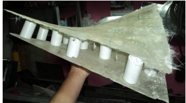
Fig. 39. Sandwich Panel W3-i. Parabolic Core PVC pipes.
