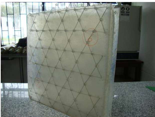
Fig. 24. Sandwich Panel W3-i. Inverted open.
