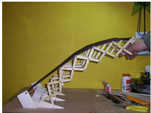
Fig. 06 Model of eccentric scissors system with membrane.
