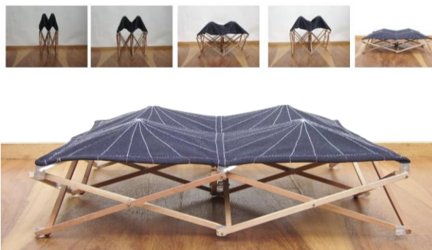
Fig. 10 Model with stiffening membrane system.
